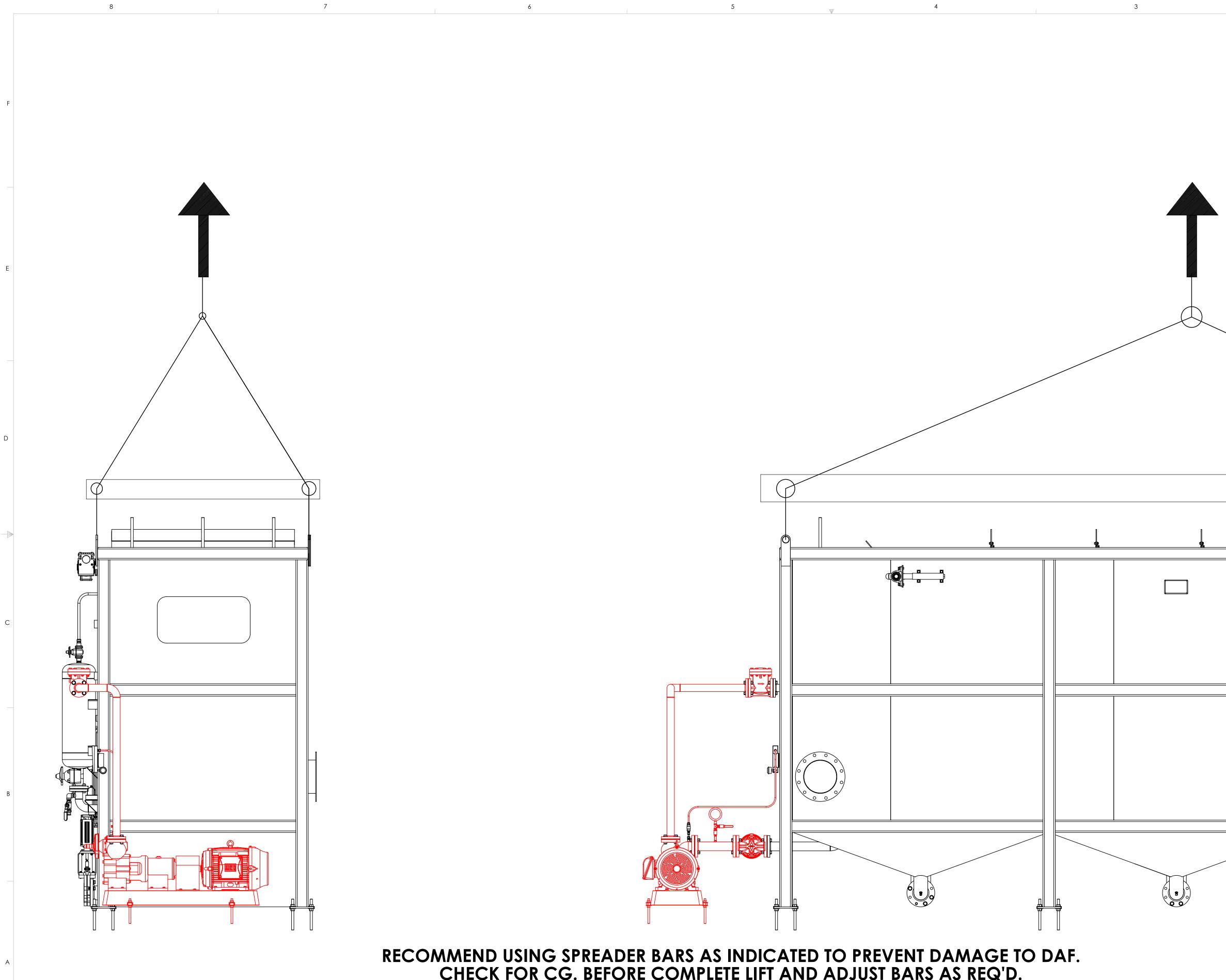
CHECK FOR CG. BEFORE COMPLETE LIFT AND ADJUST BARS AS REQ'D. ITEMS IN RED SHIPPED SEPERATELY FROM DAF, INSTALLED IN FIELD. ESTIMATED DRY WEIGHT: 13,700 LBS.
