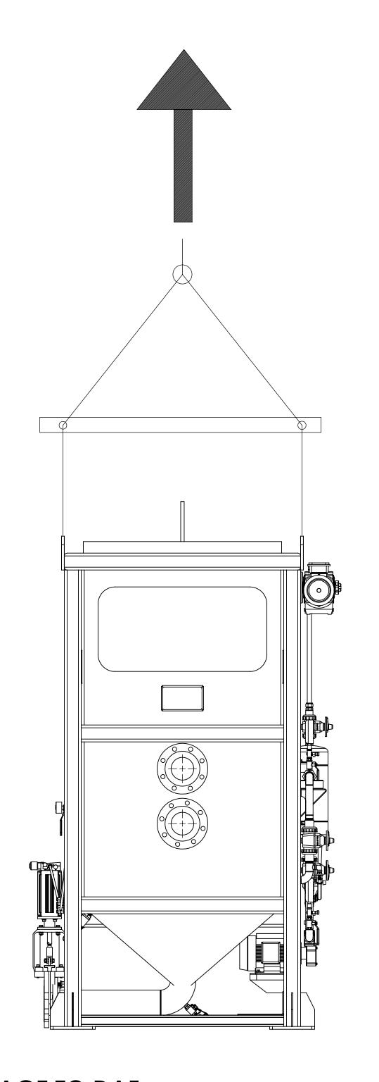
RECOMMEND USING SPREADER BARS AS INDICATED TO PREVENT DAMAGE TO DAF.
